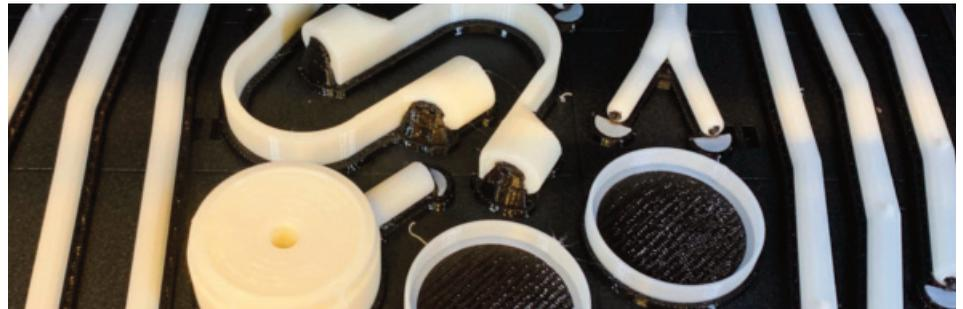
3-D Printed Face Shield Components
