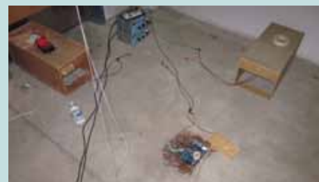
A view up the drop shaft. Students Alan Reed and Matthew Luchette constructed an electronic project as part of Dr. Mark Stewart's PHYS 241 course, Basic Electronics. Their device provides a pendulum in the Sci-Tech drop shaft with enough of a kick at just the right time for the pendulum to continue to swinging indefinitely.
