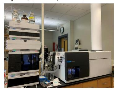
Agilent LC/Q-TOF Mass spec is located in the Instrumentation laboratory workspace in Science & Technology lab 262.
