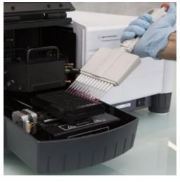
The *Agilent Cary Eclipse Fluorescence Spectrometer* with micro well plate reader is located in the Bio and Macromolecular Chemistry laboratory workspace in **Science & Technology 361**.
