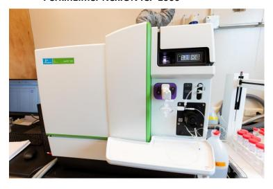
**The NexION® 1000 ICP-MS** is located in the **Instrumentation laboratory Science & Technology 262.**
