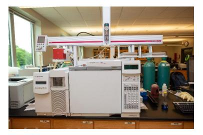
Agilent Gas Chromatography Mass Spectrometry (GC/MS) is located in the Analytical laboratory workspace in Science & Technology 262.
