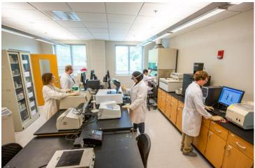
The **Biochemistry laboratory** is a spacious and highly ventilated workspace in Science & Technology 361-362. Some fixed features include a walk-in cold room, two class A fume hoods, and a biosafety level 2 cabinet.
