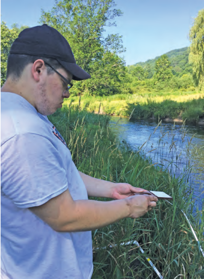
Cole Davis using a device called a densitometer. Cole measured the canopy cover at the field site (i.e., how much of the location is covered by shade from trees). Photograph by Emily Rollinson.
