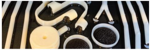
3-D Printed Face Shield Components
